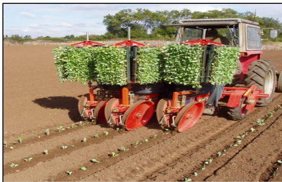
Figure 2. A Transplanter attached to a tractor transplanting seedlings
